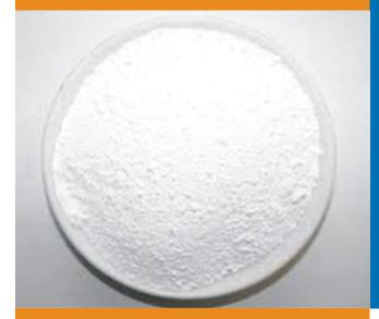
MEOS is a supplier of Barite as per API 13 A specifications. Barite is the most popular weighing material used in drilling applications. MEOS supplies Barite of Specific Gravity 4.2 (as per API requirements), 4.15 and also 4.1 specific gravity.
